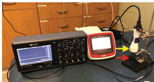
Figure 1 —Image of the custom jig (right) constructed to hold a laser probe (yellow arrow) to the surface of each anatomic site of interest and to hold a photodiode (PD; red arrow) exactly 90° to the laser beam and in contact with far surface of the site when evaluating class IV laser penetration through tissues of 20 nonsedated client-owned dogs between October 1, 2017, and December 1, 2017. The PD was attached to an oscilloscope (left) for signal detection.
